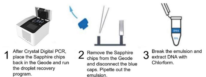
**Figure 1 | Overview of protocol of amplicon recovery from the Sapphire Chip.** The recovery and extraction procedure take less than one hour for up to 24 samples.
