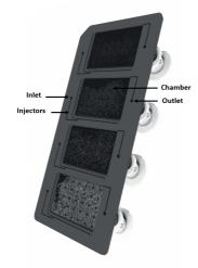
(https://cdn.technologynetworks.com/tn/images/body/sapphire\_chip\_stilla1509112338722.png)At this stage, the Sapphire chip undergoes temperature cycling to achieve DNA amplification and RNA analysis through PCR, as well as whole genome amplification. Stilla uses a fluorescence reader to quantify signals from three channels, and proprietary software to obtain concentration readings.
