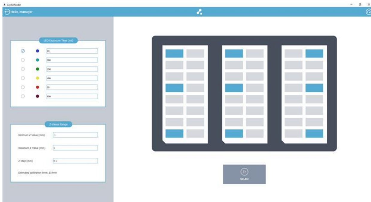
Figure 30: Example of selection of nine chambers to calibrate the focus for the Opal chip in the Crystal Reader software.
