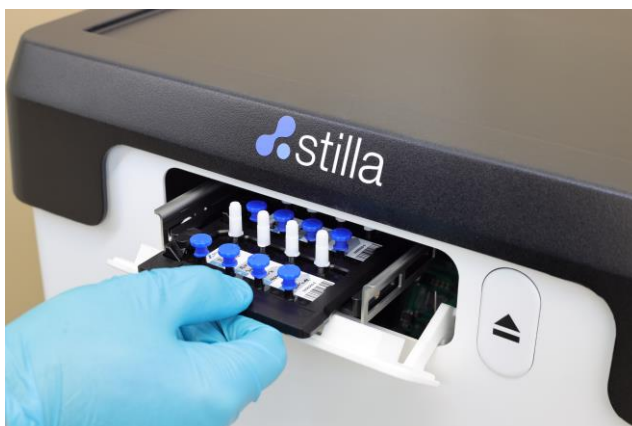
Figure 3: Fully ejected position of the moveable tray. In this position, the moveable tray is ready to be loaded with the tray holder for chip scanning.
