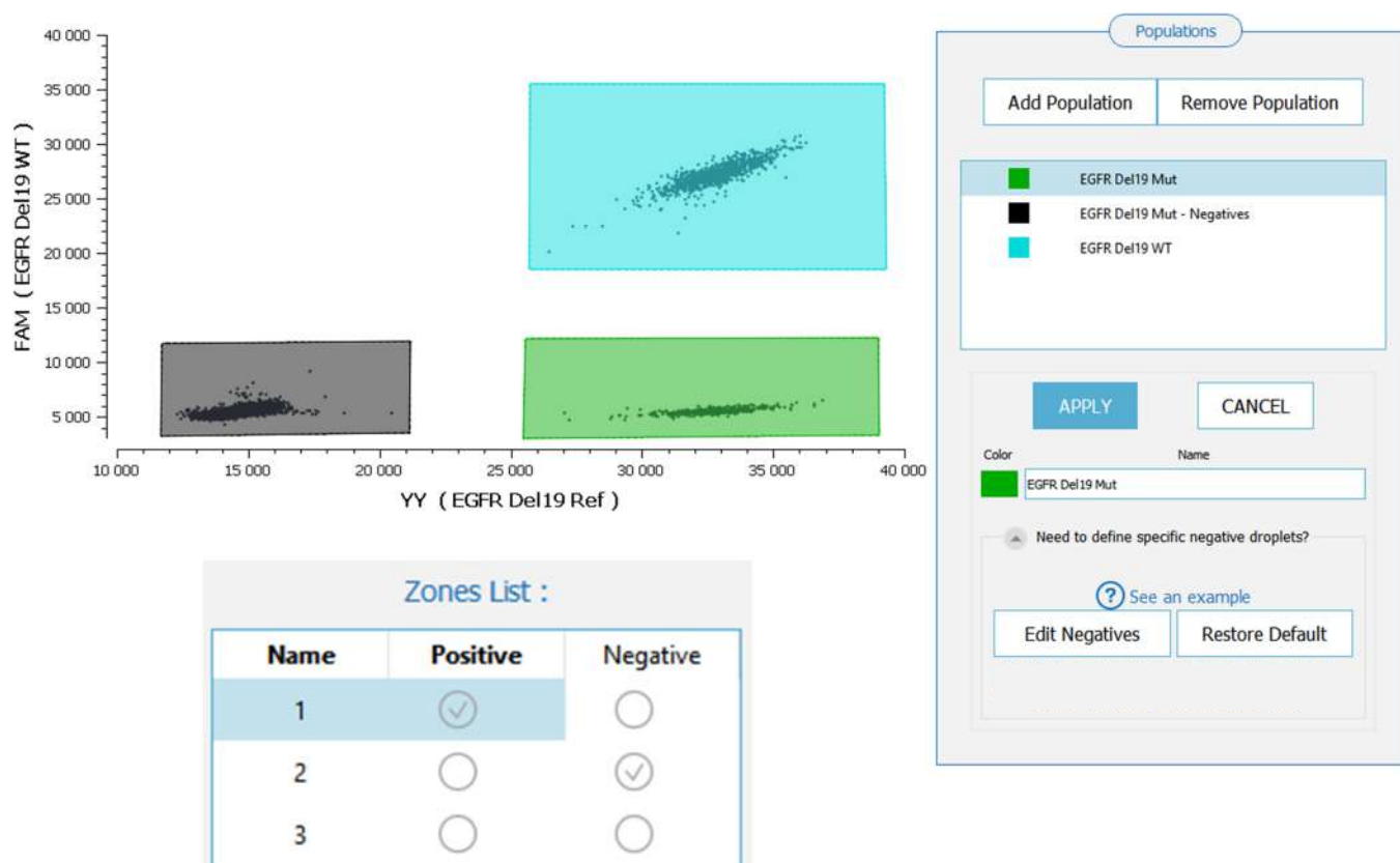
Figure 2: Example of Crystal™ Miner’s display for a digital PCR experiment targeting the drop-off mutant EGFR Del19 using two channels (channel 1: reference probe with YY fluorophore; channel 2: drop-off probe with FAM fluorophore). In the case where the 3rd detection channel is used, for example to detect an unrelated mutation or an internal control, the polygon zones will project in the 3rd dimension so they may contain droplets that are negative or positive for the 3rd detection channel. The use of a 3rd channel will in no way impact reliable drop-off quantification.
